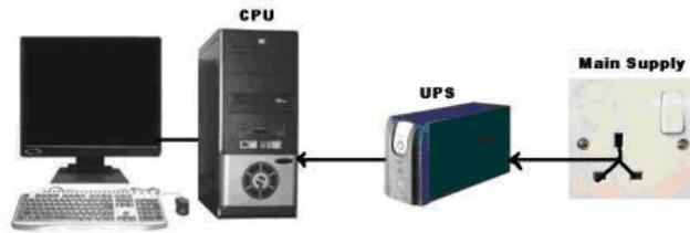
**Fig. 3.1.1 -connecting computer through UPS**
