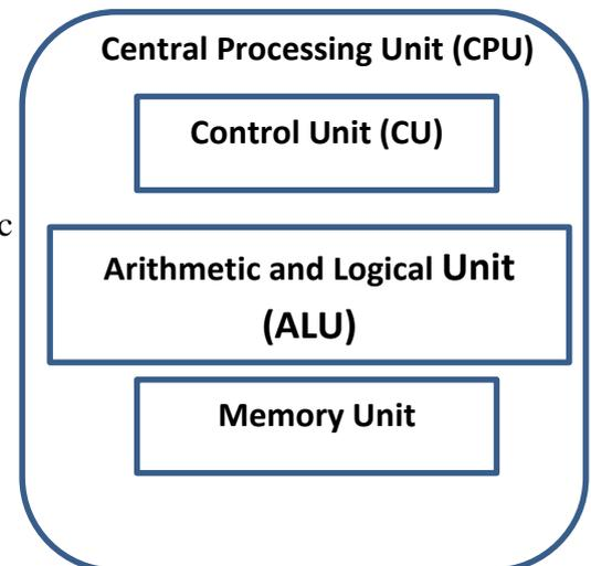
Fig. 1.1.2 - Components of a CPU
